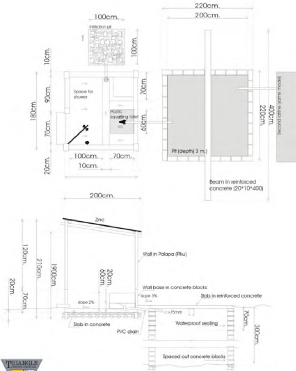
Drawing for double pour flush latrine with common pit.
