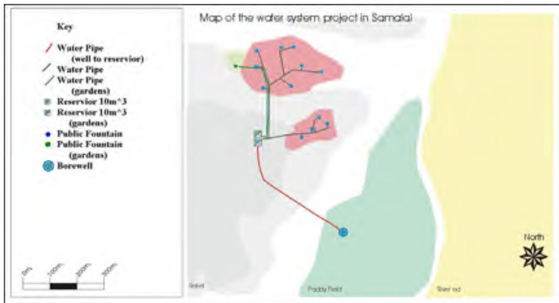
**Figure 7: Water production and distribution system in Samalai, East Timor.**
