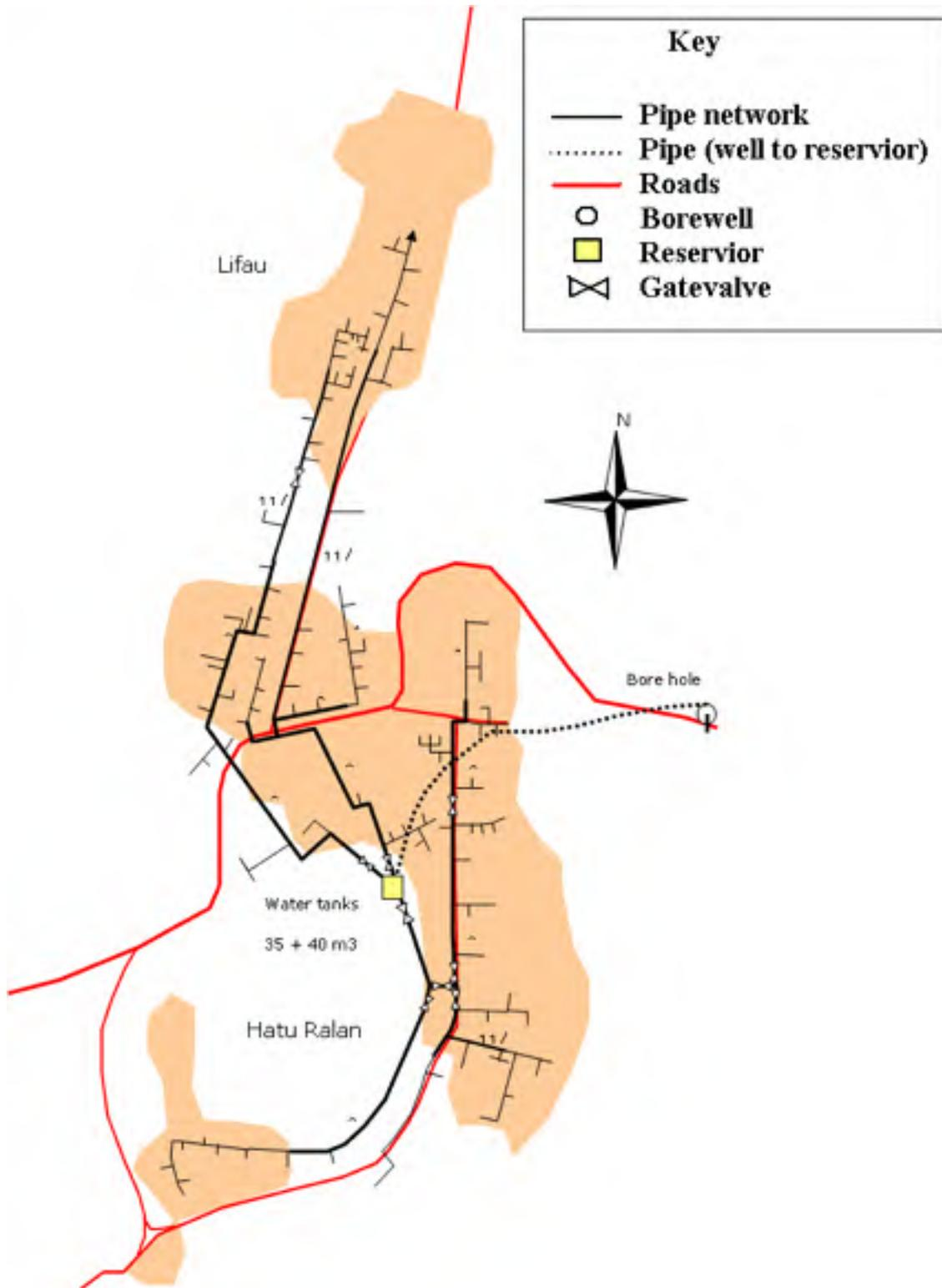
**Figure 5: Water production and distribution system in Laleia, East Timor.
