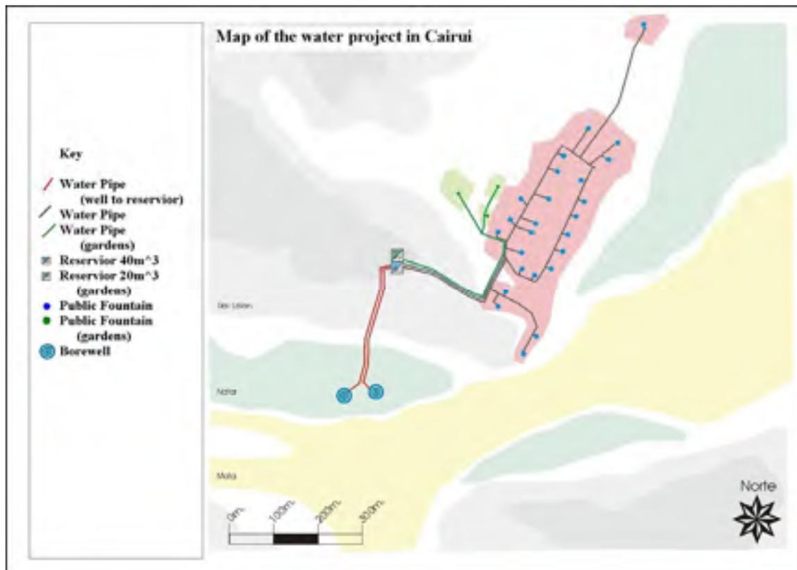
**Figure 8: Water production and distribution system in Cairui, East Timor.**
