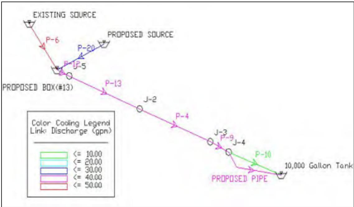
**Figure 4-2 : Schematic of system with new source and use of junction box to unite flows from two sources for a community of 150 houses. An additional pipe was deemed necessary in the lower reaches of the conduction line before the tank to carry the additional flow from the new source, partially due to the junction box acting as a pressure-break tank.**
