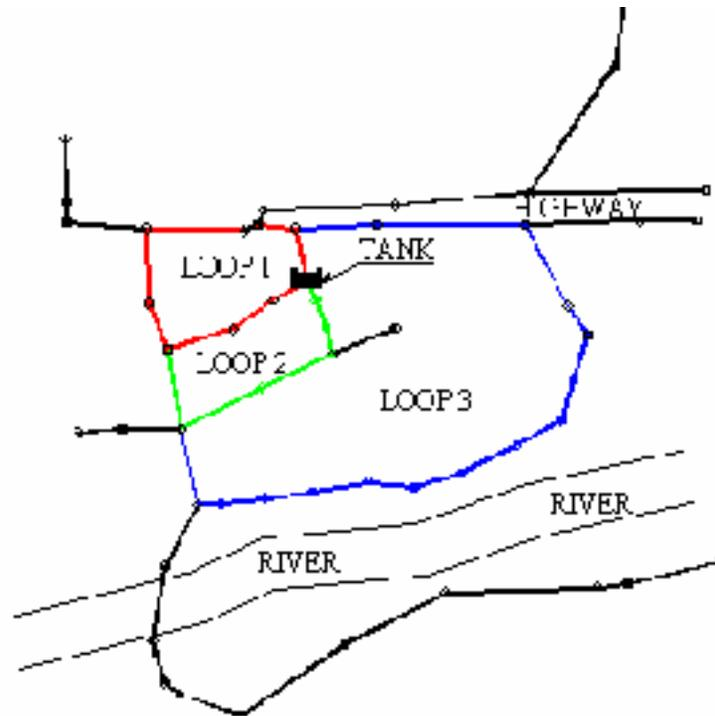
**Figure 4-9: Planimetric view of system with 3 loops for community of 70 houses, providing multiple paths for water to arrive to many sections of the community. All tubing is of 2" diameter for ease of construction.**
