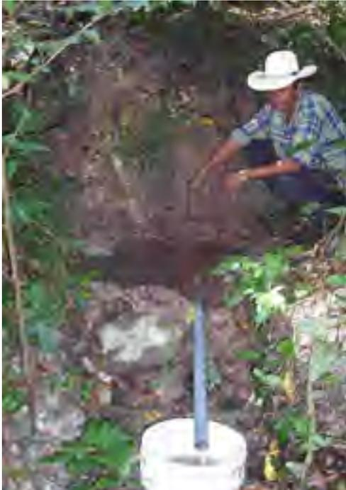
**Photo 11: Water quantity is measured at the source**
